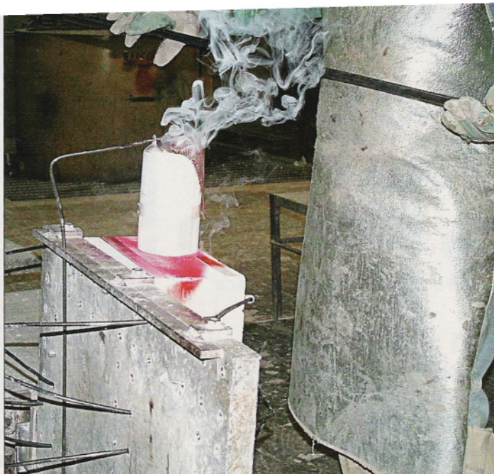
The plaster molds are gravity-poured in either A356 aluminum alloy or ZA8 zinc alloy. The molds' porosities help produce parts with uniform densities.
